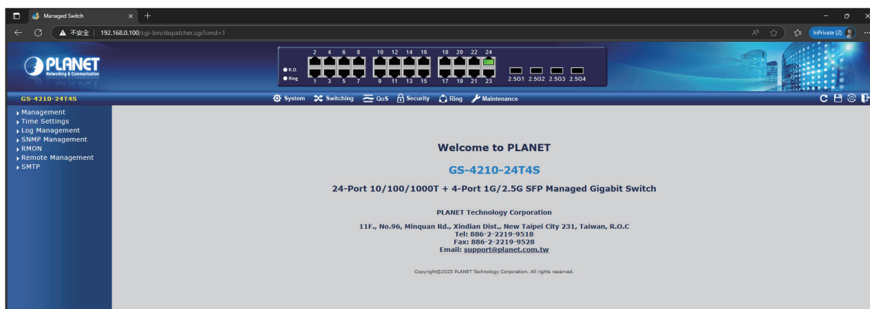
Figure 4-6: Web Main Screen of Managed Switch
